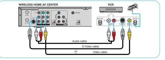
Connect the Video/Audio cables between the VIDEO or S-VIDEO / L - AUDIO - R jacks to the WIRELESS HOME AV CENTER and VIDEO or S-VIDEO / L - AUDIO - R output jacks on the VCR. (Note: For better video, use an S-Video cable.)
